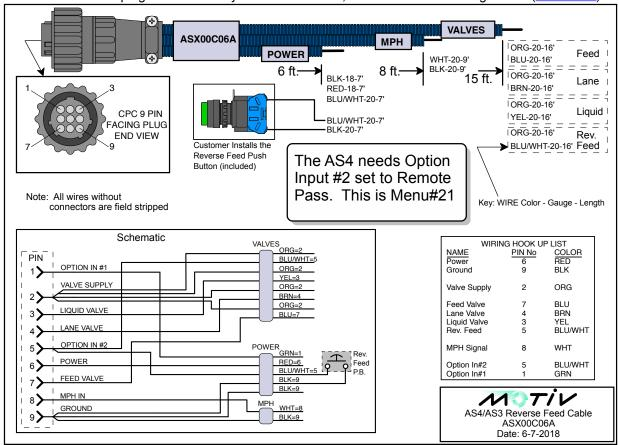
**Optional Panel Mount BracketAS4 Wiring diagram**
