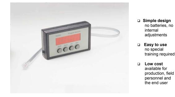
The RD200 is a small handheld display and keypad module. It plugs into the SPI port of a *Motiv* controller for viewing or editing program information. The RD200 allows the installer to quickly set up an electro-hydraulic controller with variables like; PWM frequency, valve drive minimum and maximums, ramp, etc.
