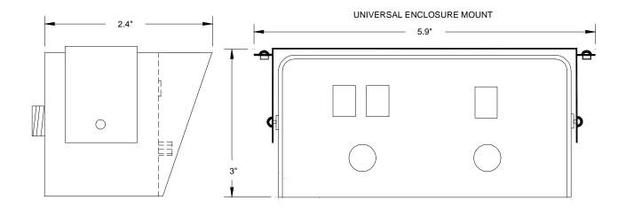
UNIVERSAL MOUNTING BRACKET PROVIDES (3) CONFIGURATIONS
